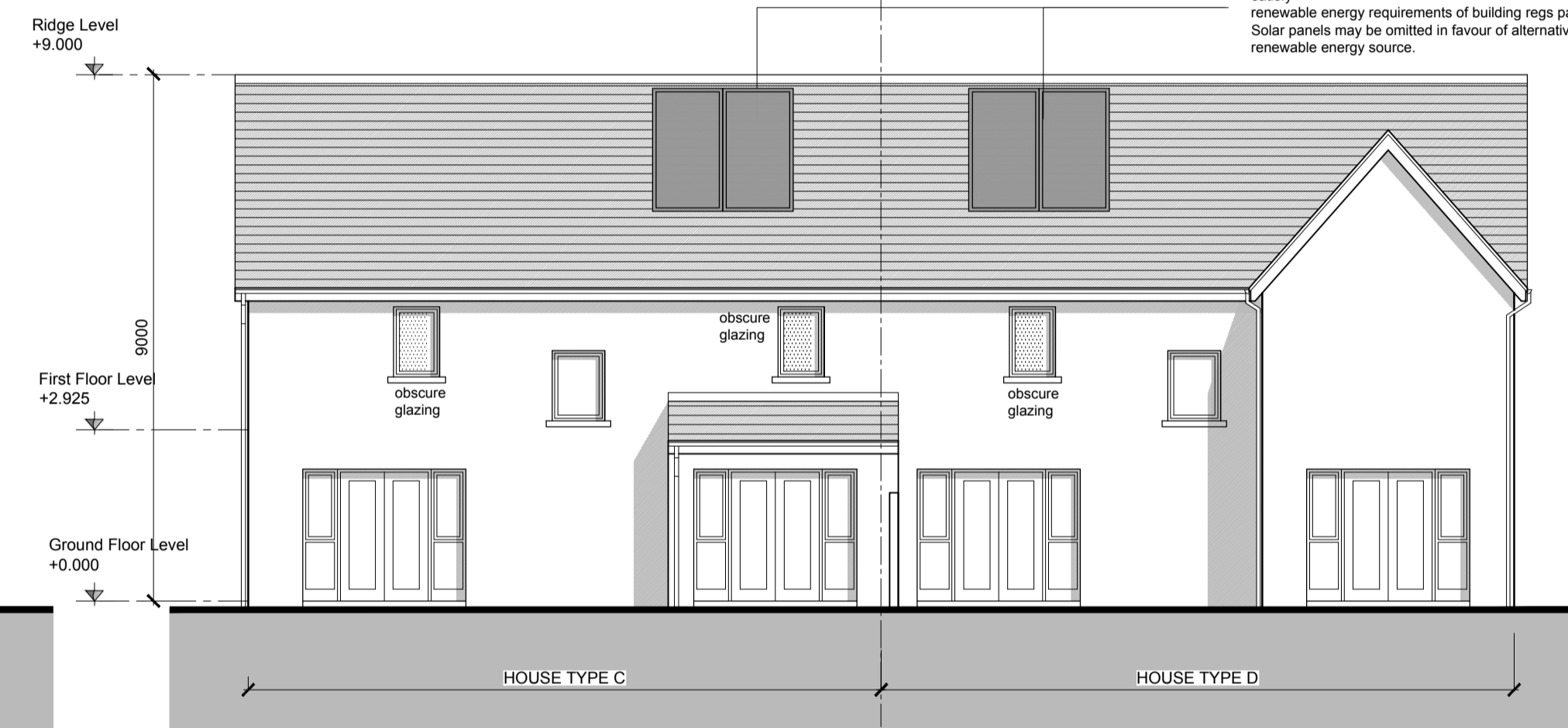
REAR ELEVATION House Type C - Semi-Detached
